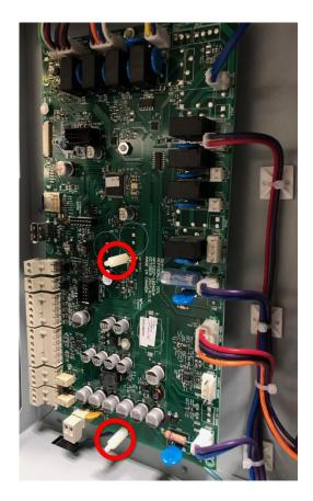
**2.2.** Place the bracket of the LonWorks FTT Module (supplied) onto the newly added nylon standoffs and secure the module firmly in place by using the nuts set aside in the previous step.
