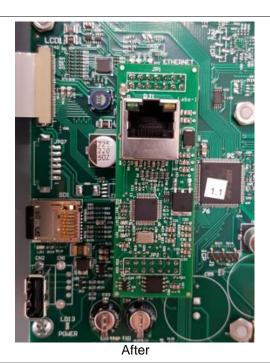
**2.4.** Connect the USB cable (supplied) between the LonWorks FTT Module and the printed circuit board, using the USB port located on the left side of the humidifier PCB. Connect the Ethernet cable (supplied) between the LonWorks FTT module and the Ethernet IP board, using the Ethernet connection located on the Ethernet board.
